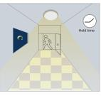
After last detection, the light will be dimmed down to the stand-by dimming level (10%, 20%,30% or 50%) after holdtime.
